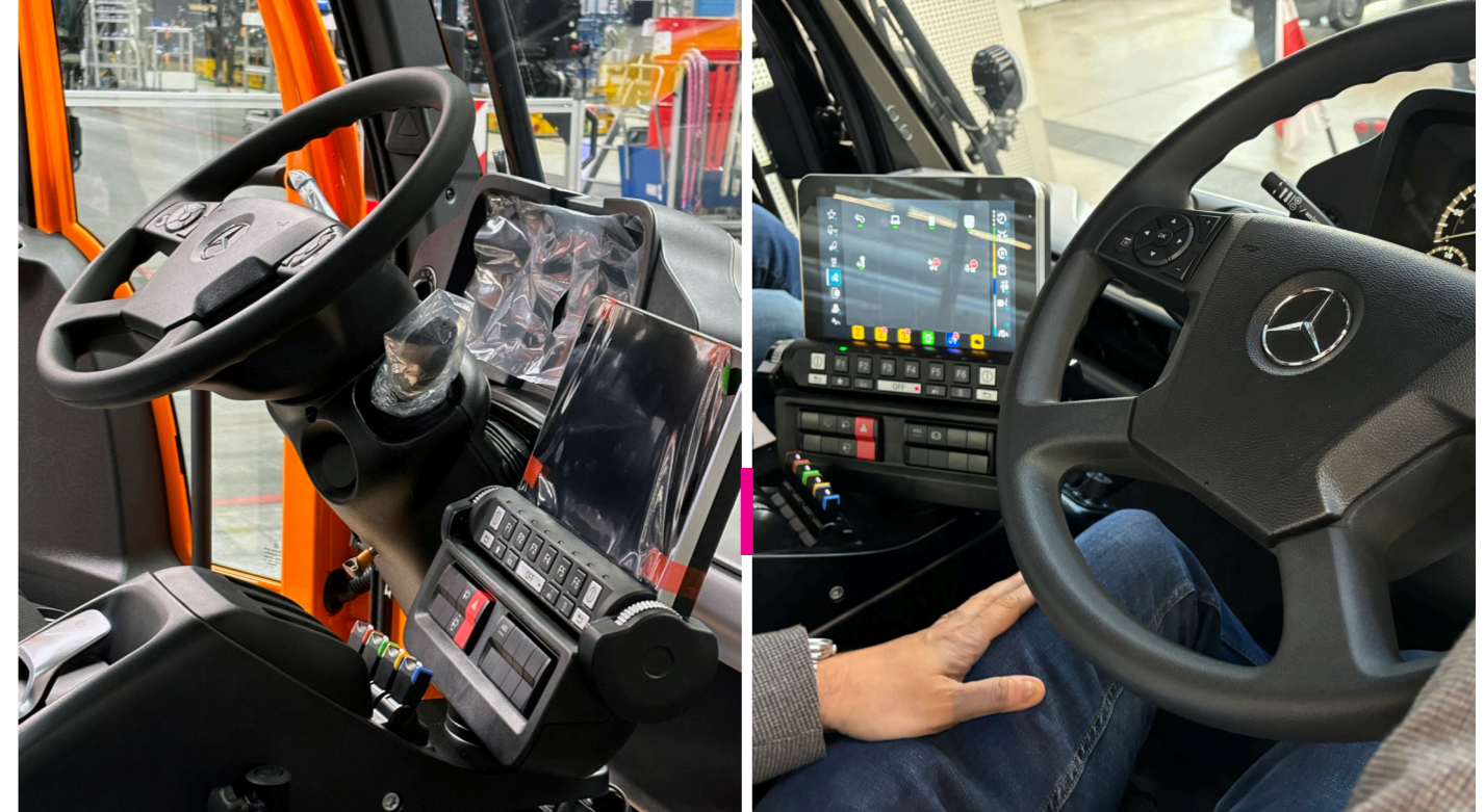
Maximum driving freedom: Installed as standard on the left-hand driver’s side, the steering wheel can be shifted to the right using a sliding mechanism.
