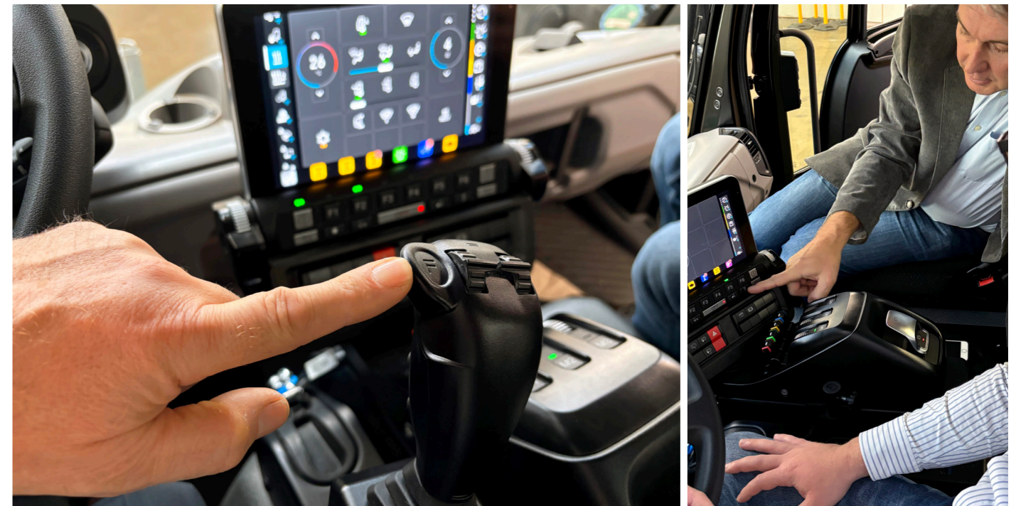
The UNI-TOUCH system at a glance: The center console features a touchscreen along with additional analog pushbuttons, various toggle switches, and the RAFI LINEAR JOYSCAPE.
